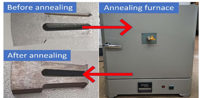
Fig. 12. (Color online) Annealed samples and schematic diagram of the annealing furnace.
