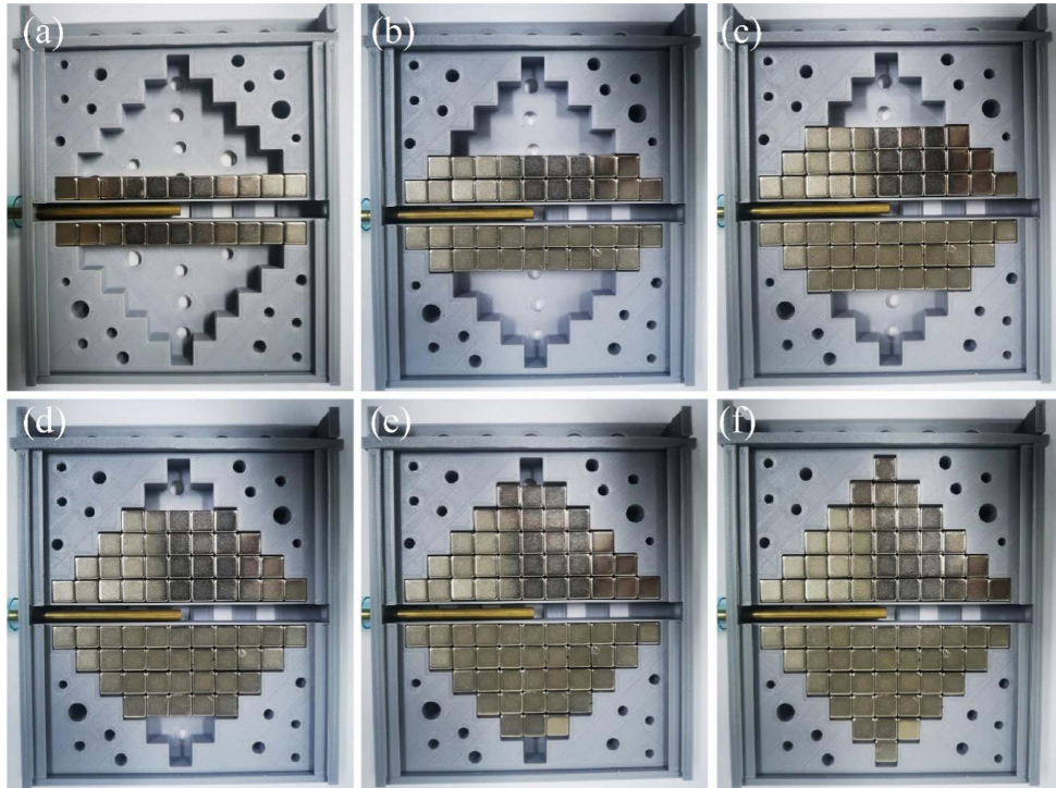
Fig. 4. (Color online) Physical prototypes of the multilayer gradient-compensated magnet configurations: (a) one layer; (b) two layers; (c) three layers; (d) four layers; (e) five layers; (f) six layers.
