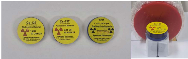
Fig. 4. (Color online) Three Cs-137 sources were stacked for the experiment, and the sources were placed at the central height of the detector to ensure measurement accuracy.
