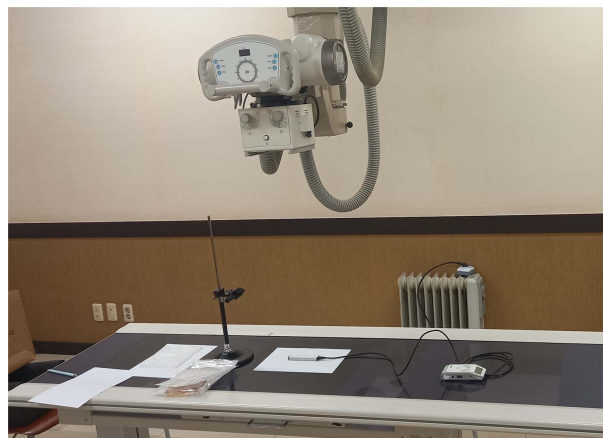
Fig. 2. (Color online) Photo of the custom-fabricated hydrogel shielding performance evaluation device for medical X-ray shielding.
