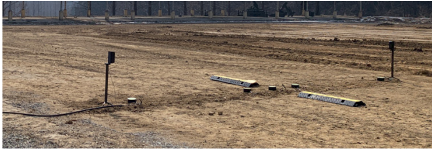
Fig. 4. Photograph of the installed measuring system for the measurement of magnetic and vibration signals from tanks and magnetic mine clearing apparatus.
